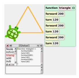
Figure 1. A screenshot from the TileScript system. The smae code is shown as tiles and text-based code.
